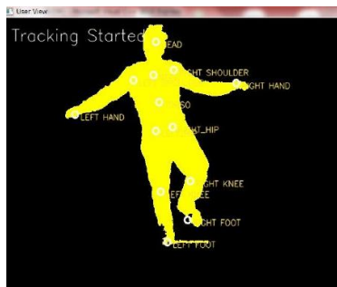
Fig. 7 An captured image and position information of user’s exercise by Kinect
