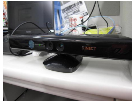
Fig. 6 The Vision System of Robot System, Kinect manufactured by Microsoft
