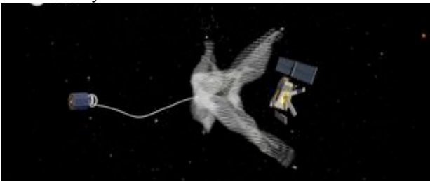
Figure 7: an e.Deorbit satellite capturing a debris (defunct spacecraft) with a throw net.
