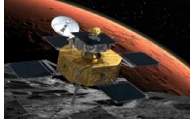
Figure 4: rendering of the Phootprint elements on Phobos. The Earth Return Capsule (ERC) is secured on the Earth Return Vehicle (ERV) which sits on the lander module. The lander module is quipped with a robot arm.
