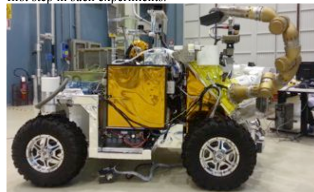
Figure 6: The Eurobot Ground development Prototype (EGP), equipped with the DEXARM robot arm, the CTED tool exchange device and the DEXHAND anthropomorphic gripper.
