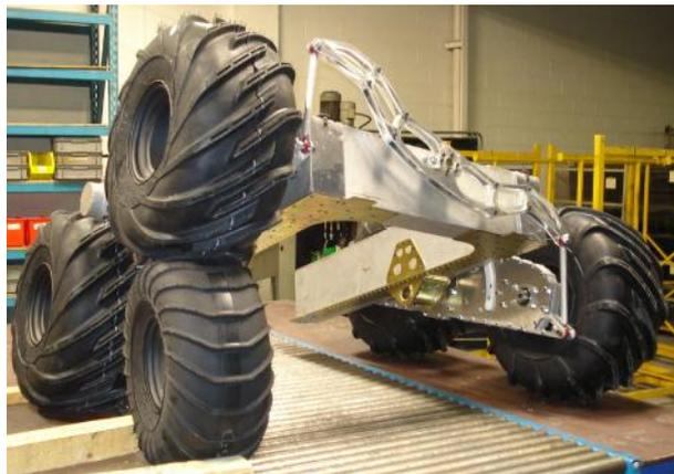
**Figure 3. Juno II suspension-arm in ‘vertical’ articulation**
