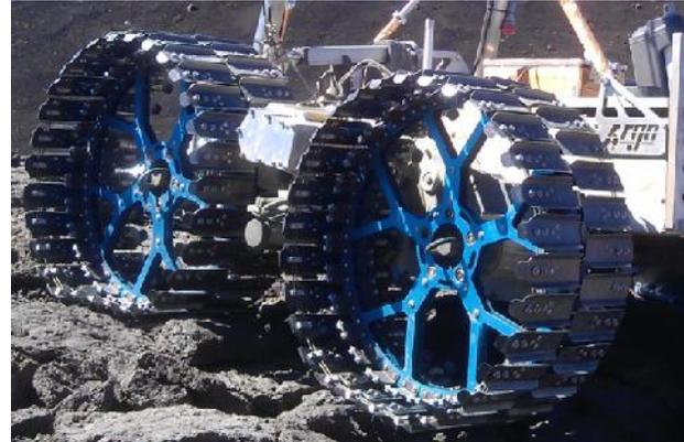
**Figure 5. TIRELESS GEN2 metallic wheels (patent pending)**
