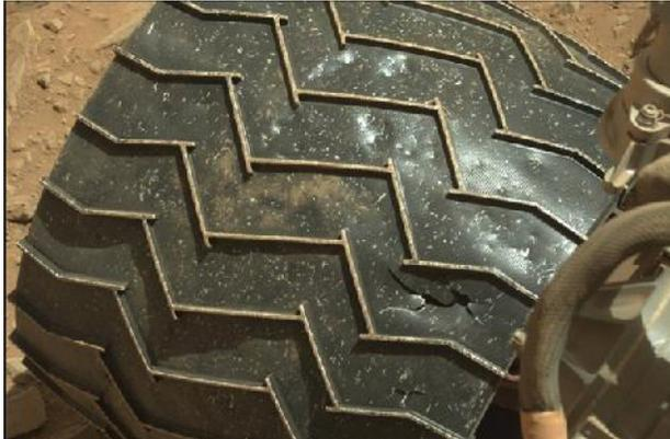
Figure 6. Curiosity wheel damage (credit NASA)
