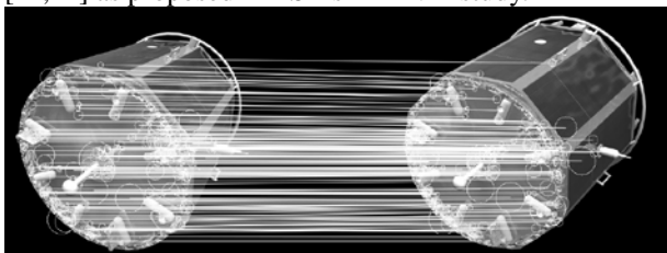
Figure 9: Results of matching of keypoints between a real object (left) and a virtual image (right).
