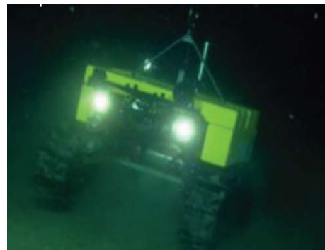
Figure 3. Deep-sea crawler in operation with data and power umbilical
