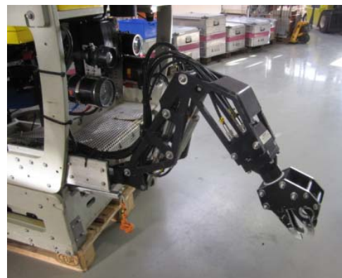
Figure 10. Manipulation by robotic arm: deep sea scenario for precise geophone placement
