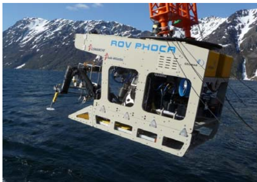
Figure 2. ROV PHOCA with 2 robotic arms
