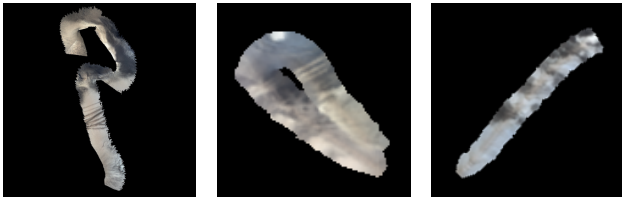
Figure 4. : Images of Traverses 1, 2, and 3 and their true location in the orbital map. Note in all three of the navcam paths there is a large amount of high frequency detail not present in the orbital map, making registration difficult. Traverse 3’s registration accuracy also suffers because it matches well with much of the local terrain.
