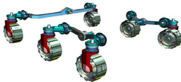
Figure 2: MDA’s ExoMars Suspension and Locomotion Design
