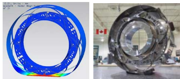
Figure 6: Wheel simulation results and MDA flexible wheel prototype
