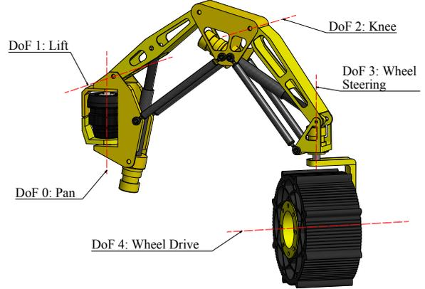
**Figure 5.** New leg design for Sherpa based on two serial aligned parallel kinematics
