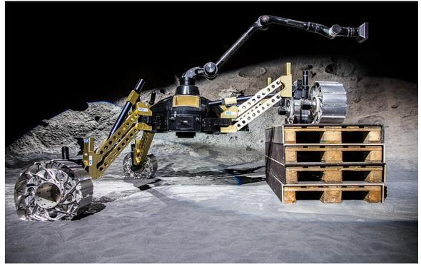
**Figure 2.** Benefits of negative ground clearance: Sherpa stepping onto a high obstacle. The manipulator was used to support the rover while lifting the wheel onto the obstacle.
