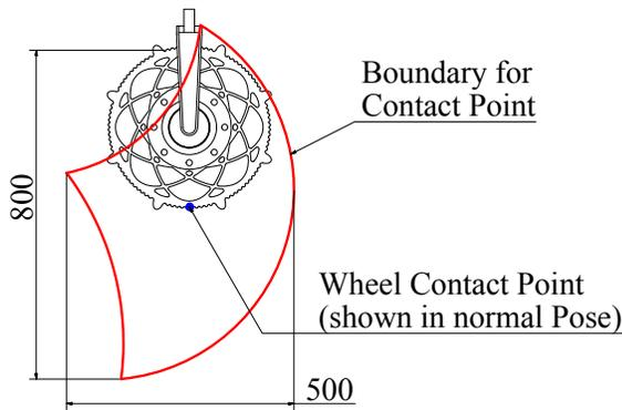
**Figure 7.** Movement range for the wheel contact point using DoF1 and DoF2. DoF0 has a movement range of  $\pm 135^\circ$  that creates a toroid of the denoted cross section. Normal pose denotes the expected nominal driving position (WCP in center of movementrange) in cross shaped stance. Dimensions are in mm.
