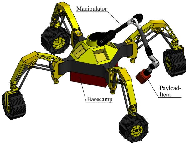
**Figure 6.** New rover suspension design. The suspension is shown in the normal pose: A cross shaped suspension alignment and at medium body height.
