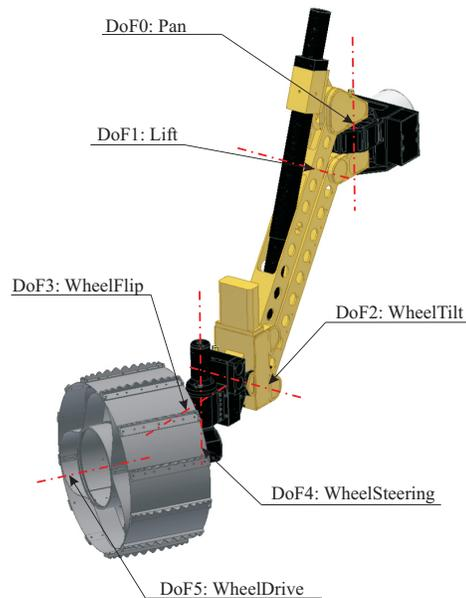
**Figure 3.** One leg of Sherpa's suspension system with numbering and naming of the degrees of freedom.
