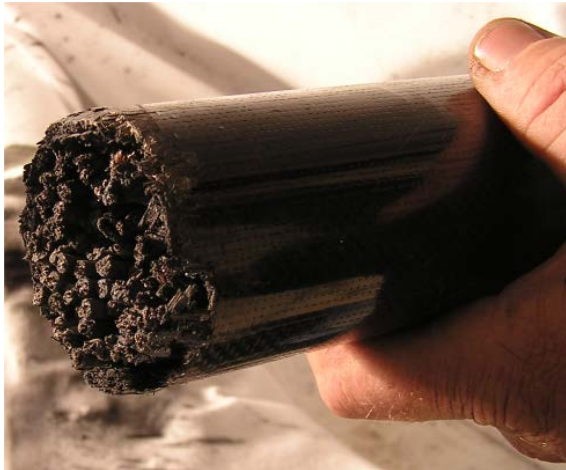
Figure 14: Cutting Result of a Carbon Fiber Tube
