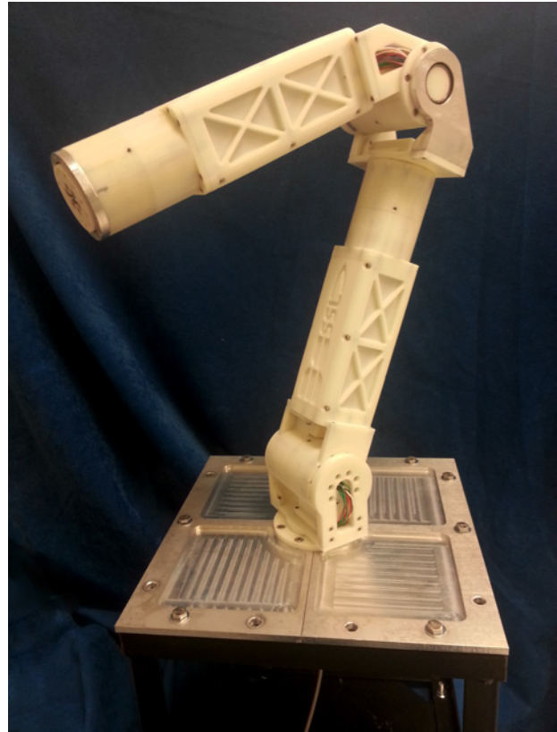
Figure 6. The DYMAFLEX high performance 4 DOF prototype manipulator
