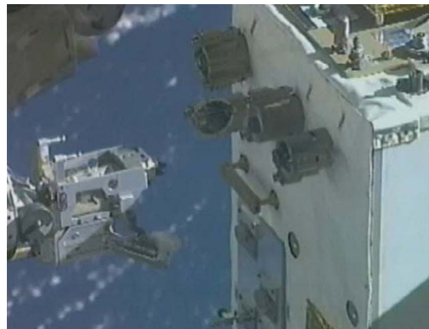
Figure 3: MFT positioned to acquire adapters for CVT1 operations (photo credit NASA/CSA)
