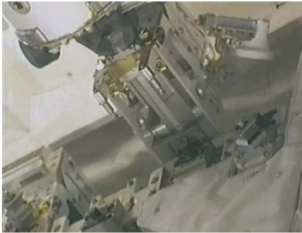
Figure 2: One of the RRM tools being removed from the RRM ToolBay
