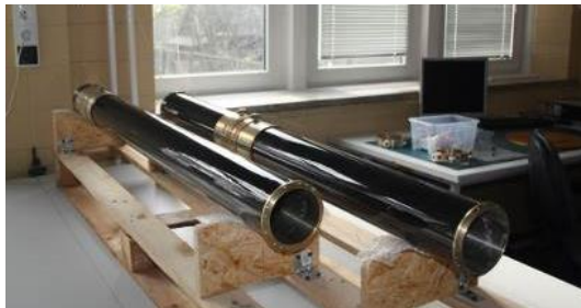
Figure 10. Manipulator links made of high modulus carbon fiber reinforced materials with interfaces and attachment for tests-bed systems
