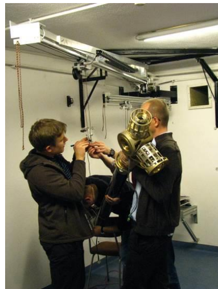
Figure 1. Prototype of robotic arm WMS1 LEMUR during integration on the suspension test-bed.
