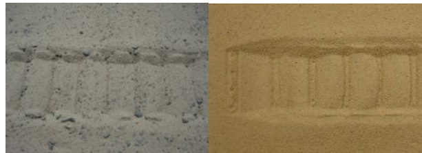
Figure 11. EXMB2 wheel track on soil ES3-OMR at 25% slip, left with and right without admixed gravel
