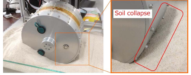
Figure 8. Snapshot view of the soil collapse phenomenon in front of the wheel
