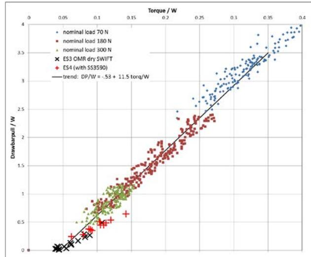
Figure 6. Graph of the correlation between torque, T, and drawbar pull, DP, both normalized after the load, W, for the 100% slip tests in UNDERSTAND, and single wheel tests in SWIFT and EXPERTISE [3], [4]
