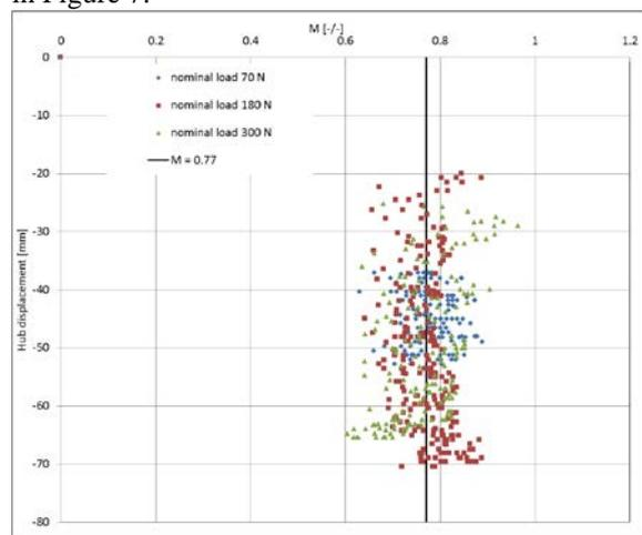
Figure 7. Graph of the sinkage and values for the parameter M (as per ‘Eq. 1’) derived from the 100% slip single wheel tests.
