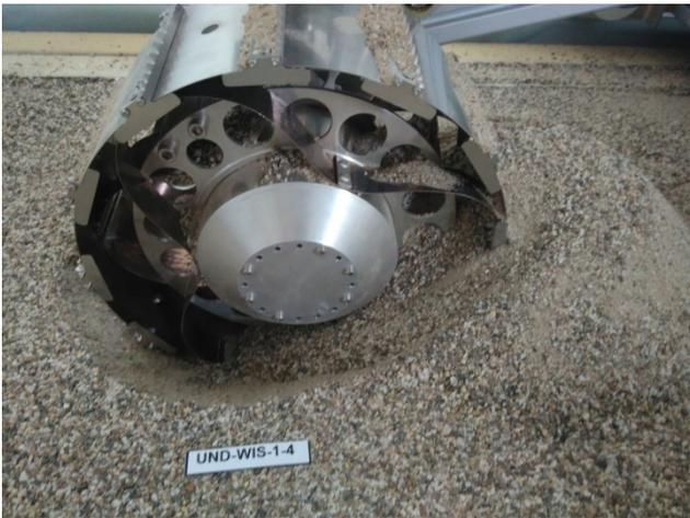
Figure 11. ExoMars phase B2 flexible wheel on Martian soil simulant ES3
