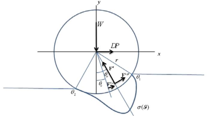
Figure 4. Sketch for the analysis of the interaction between a wheel and deformable soil during driving as used in the WPM [3].
