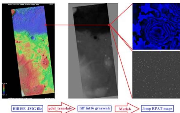
Figure 12. Example of map making process flow
