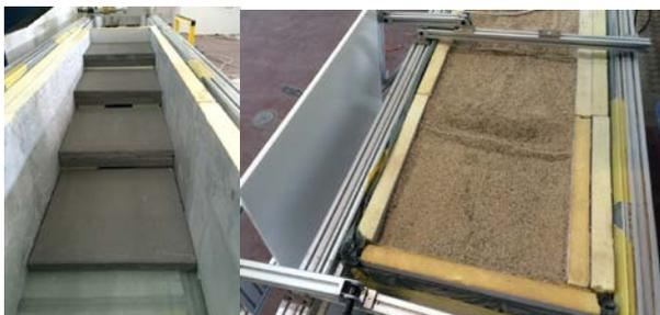
Figure 2. Set-up for measuring thermal variation with various thickness of soil layer
