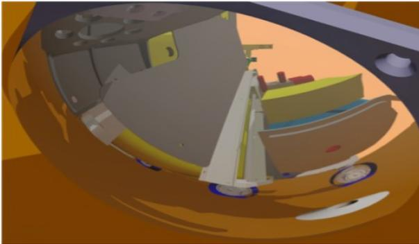
Figure 8. PanCam estimated view using the Rover Inspection Mirror (RIM)
