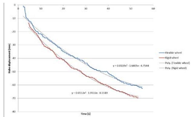
Figure 10. Sinkage measured during experiment for the ExoMars phase B2 flexible wheel and a rigid wheel of same diameter
