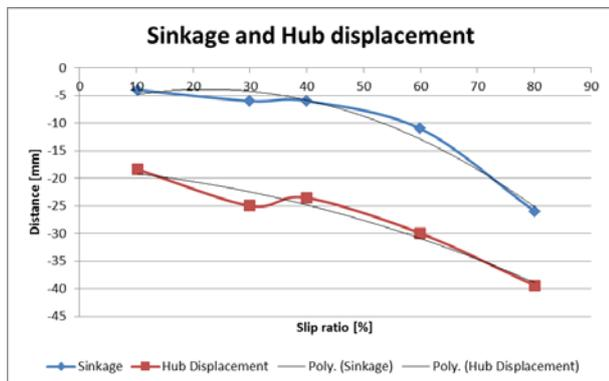
Figure 9. Sinkage and hub displacement of the ExoMars phase B2 flexible wheel as a function of slip ratio [4] Using the measured wheel radial stiffness, for the lower
