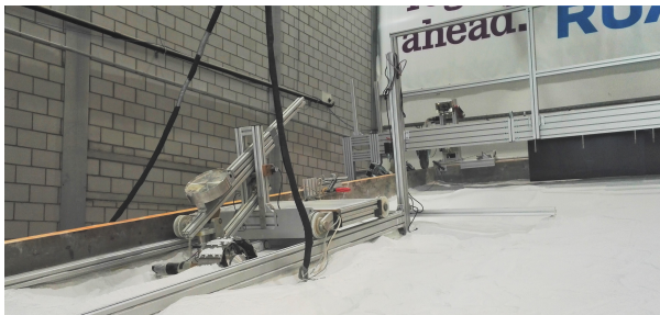
Figure 6: Tilted SWT at large slopes exhibiting high wheel sinkage. The soil below the motor was partially removed to avoid motor-soil contact.
