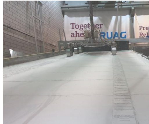
Figure 6. ExoMars LVM Gradeability Test on soil ES2
