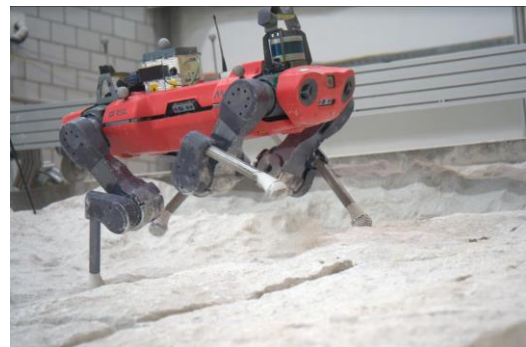
Figure 11. ANYMal test on hard bedrock. Image credit: Robotic Systems Lab, ETHZ
