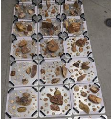
Figure 8. JPL tiles for locomotion testing
