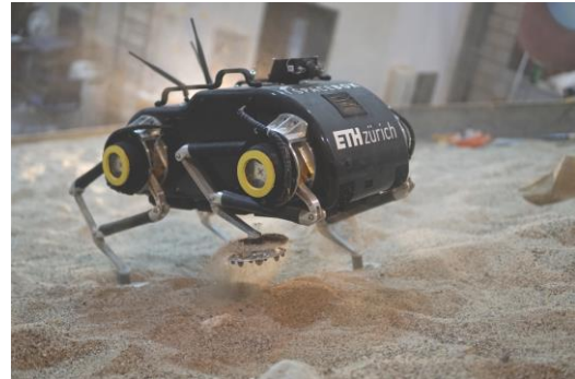
Figure 10. ETH SpaceBok gradeability test
