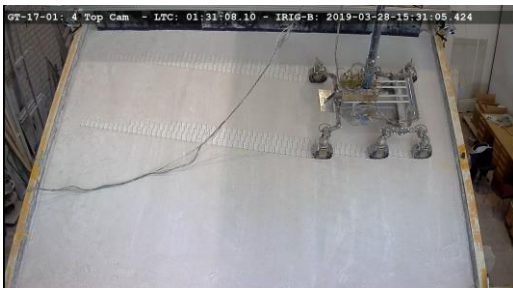
Figure 5. ExoMars LVM cross-slope on soil ES2, video including LTC and IRIG-B time
