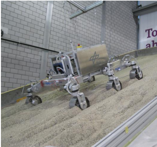
Figure 4. ExoMars B2 DLR rover - Gradeability Test on ES3
