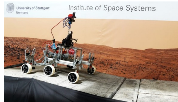
Figure 1: IRS Modular Rover Chassis Platform during testing of student designed on-board sensory packages.
