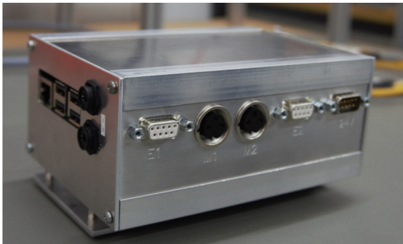
Figure 7: Electronics Box Assembly housing the OBC and motor controllers.
