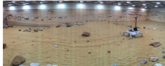
Figure 11. IBB1 testing of the GNC subsystem in the Mars Yard in Airbus facilities in Stevenage [UK]
