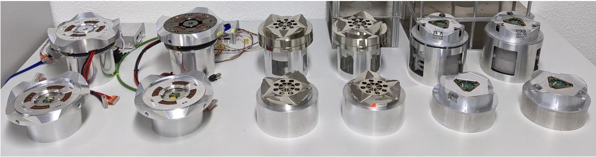
Figure 1: The used SIs with their adapters from left to right: iSSI® active and passive with optional formfits, HOTDOCK active and passive and SIROM active and passive. The passive SIs are in the front row
