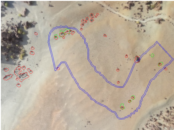
Figure 5. Tenerife final tuning results. Blue is propagated field of view, red is ground truth obstacles and green is detected obstacles.
