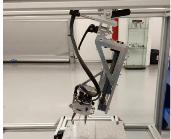
Figure 4. Gripper testing with the MGSE (courtesy of AVS)
