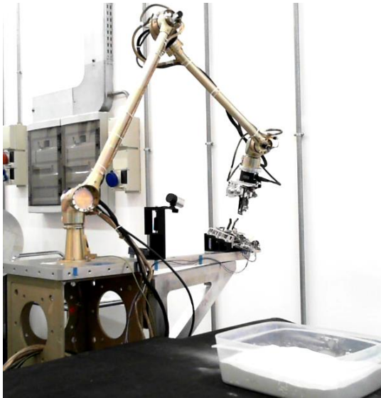
Figure 6. Testing of RRB with Gripper installed on the DELIAN arm
