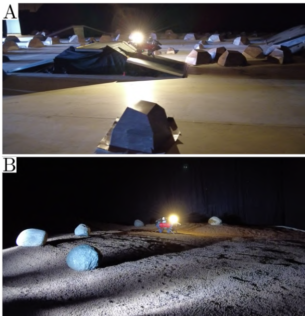
Figure 4: (A) ANYmal GLIMPSE crossing the steepest obstacle in the traverse area. (B) ANYmal GLIMPSE in the ROI. Despite the high sinkage on the granular soil, locomotion worked robustly.
