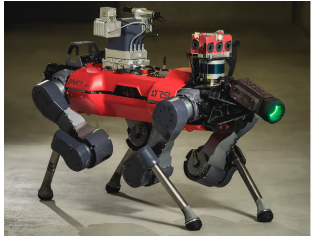
Figure 1: We equipped ANYmal with state-of-the-art sensors for navigation, mapping and localization, and a broad scientific instrument suite for resource prospection.
