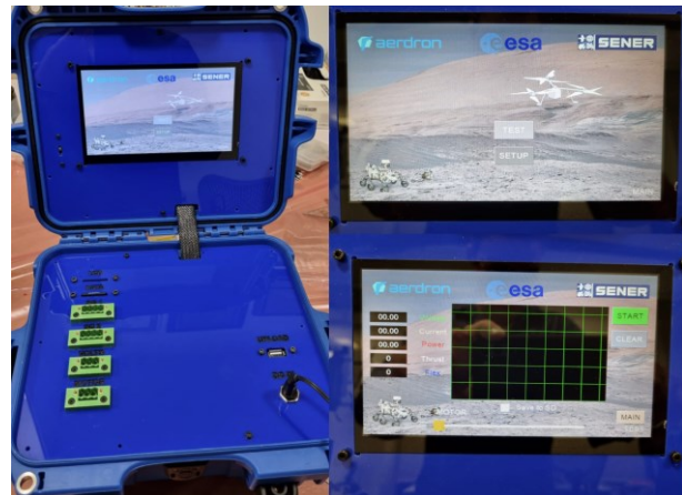
Figure 11. Propulsion test bench controller
