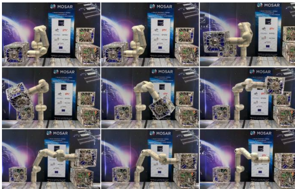
Fig. 15. Manipulation sequence of a spacecraft module from the servicer spacecraft.
