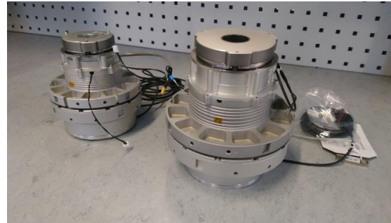
Figure 7. Robotic drive units – elbow/wrist (left) and shoulder (right).
