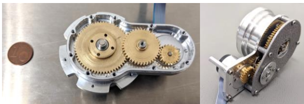
Figure 6: Development of a new type of sealed high-performance micro drive units
