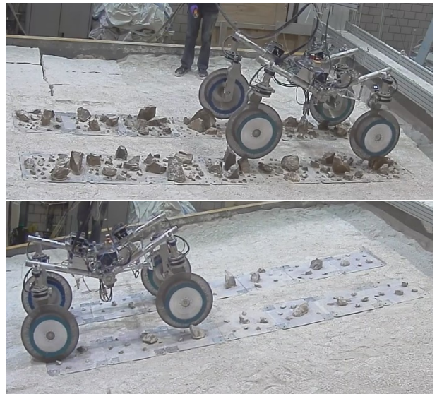
Figure 12: Terrain traversal test, Life Terrain (top) and 10% CFA (bottom)
