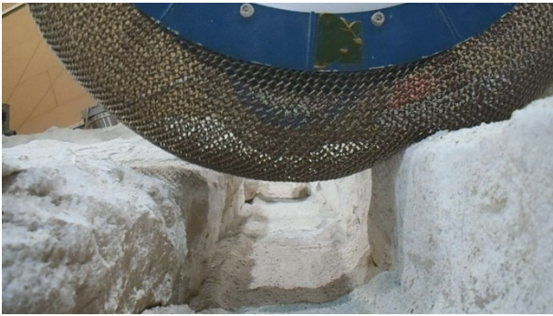
Figure 10: Wheel deformation during crevasse test
