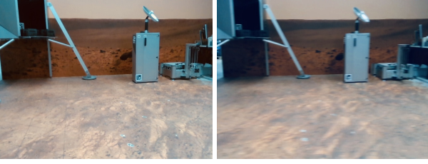
Figure 2: Exemplary images from the SurfA setting depicting the degree of motion blur to be expected within the contemplated projects. The image on the left-hand side illustrates the motion-blur-free case from dataset 11, whereas the image on the right-hand side from dataset 12 shows an increased degree of disturbance.
