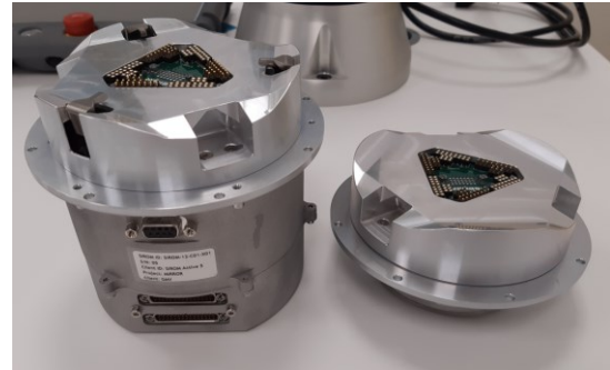
Figure 14. Active (left) and passive (right) SIROMs.
