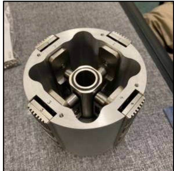
Fig. 9. The clamp unit. As with all the subsystems, a toroidal architecture was required to allow the central auger to pass through the middle.
