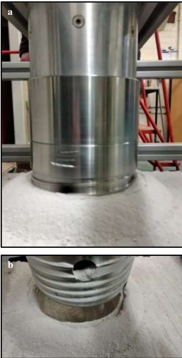
Fig. 7 (a) and (b). The cutting face proceeds into the target material, and the spoil arising is transferred into the cutting face, through the circular windows, for uplift.
