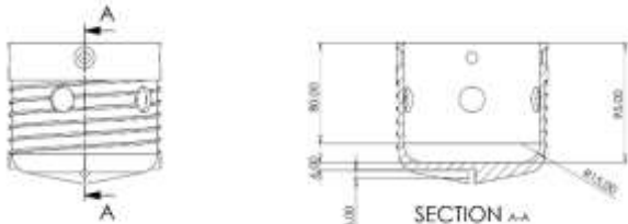
Fig. 4. The cutting face which contains the stirrer plate. A tungsten-carbide tooth (not shown) fits in the slot at the bottom, and is secured by a horizontal set-screw.
