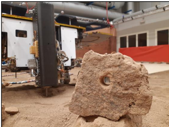
Picture 12: Drilled rock buried in the MTS terrain that allowed to de-risk the deep drilling to be performed in the drilling facility.
