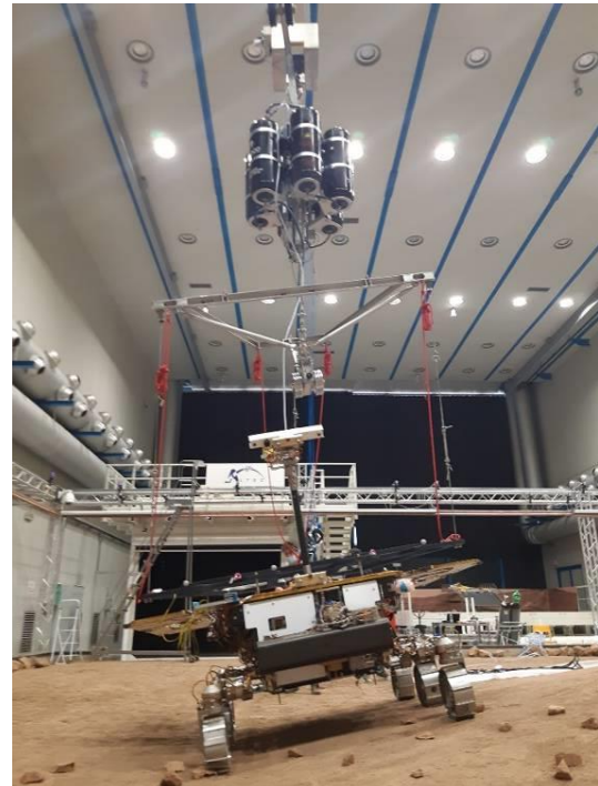
Picture 7 Amalia Rover with the Rover Unloading Device (RUD) on the Mars Terrain Simulator (MTS)
