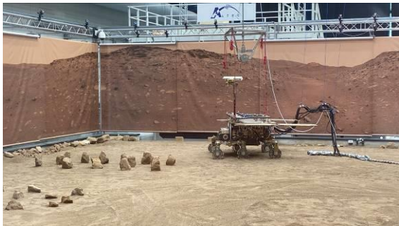
Picture 29: Amalia arriving to the target C running CNES Autonomous Navigation [14] during the confidence testing prior to SVT-4.
