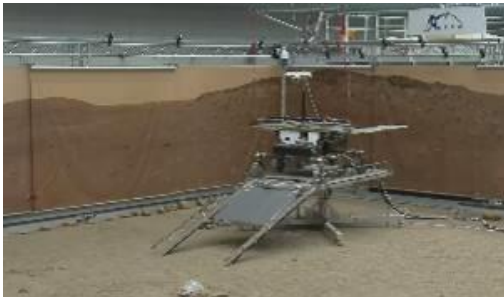
Figure 25: Rover configuration after solar arrays deployments and mobility deployment
