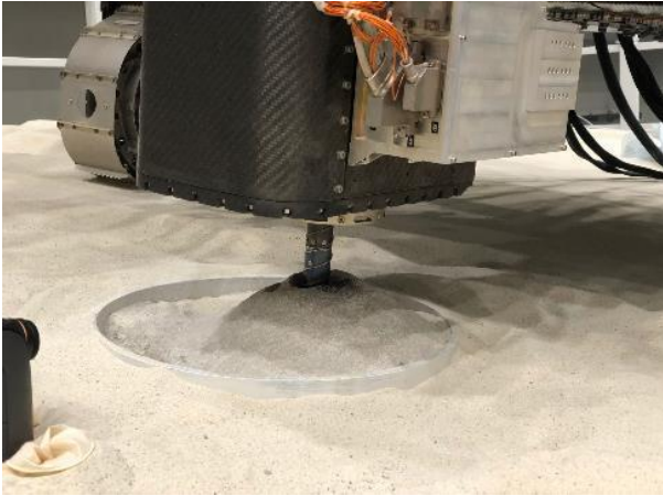
Picture 15: Drilling on-going with drill fines accumulating into a cone of material that could be imaged by the PanCam Rover Inspection Mirror (RIM) and CLUPI.
