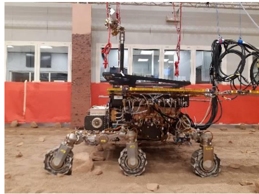
Picture 9: Amalia rover performing auto-stand-up against a rock.
