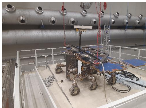
Picture 14: Amalia Rover on the drilling platform facility with drill deployed.
