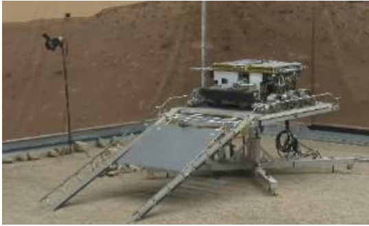
Figure 23: initial configuration at landing after ramps deployment (only the front ramps inclined of 20deg with flat floor are available on the landing mock-up)
