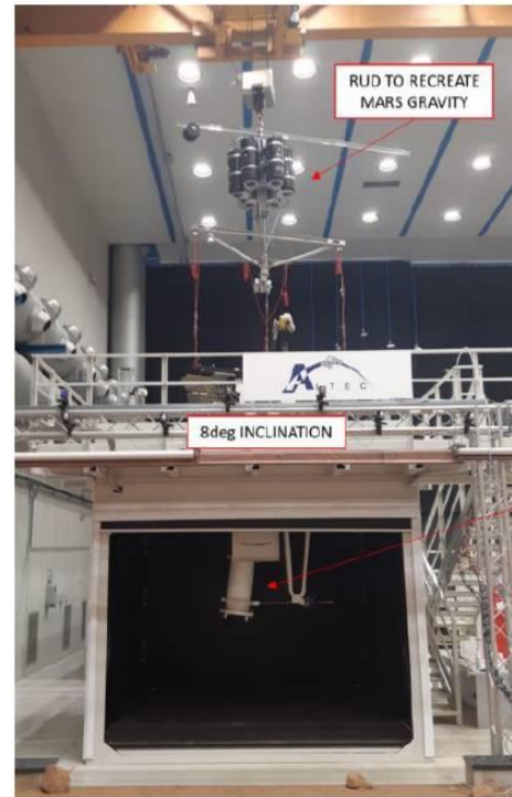
Picture 13: ROCC MTS Drilling facility with well tilted to 8deg and Rover suspended on the RUD on top of the platform.
