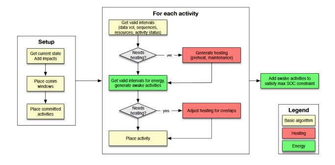
Figure 1. Onboard scheduler algorithm.
