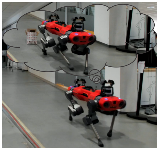
Figure 1. The high-level concept idea of an ANYmal robot with episodic memory. When in a situation the robot has previously been in and deemed important, for example due to detection of some error or anomaly, it is able to actively remember and replay this memory. This allows the robot to evaluate its situation based on this explicit past experience.
