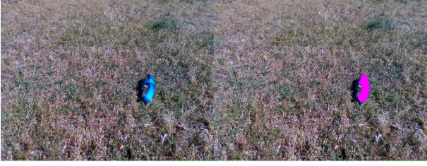
Figure 3. The anomaly detection with live data from the robot. On the left side, the input image is shown. On the right, the corresponding segmentation mask of the ensemble based anomaly detection is highlighted.
