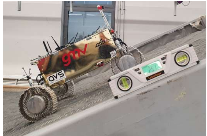
Fig. 13. EMRS tests, 25° slope, at DLR PEL
