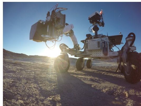
Figure 2 - MESR rover deploying mini-corer and TEMMI microscope using robotic arm during the 2015 Utah analogue mission
