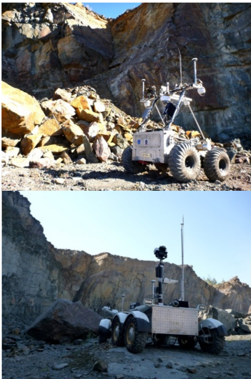
Figure 4 Artemis Jr rover (top) and LELR (bottom) during GN&C Testing
