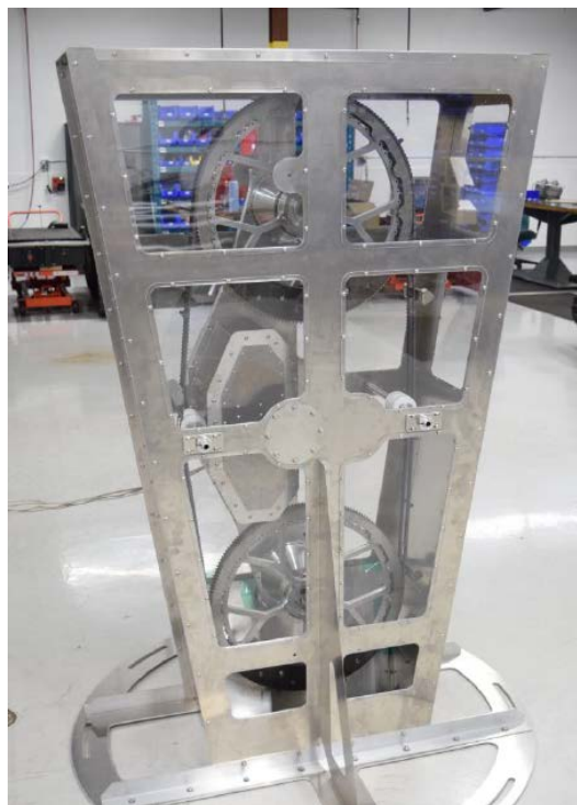
Figure 6 - LRPDP Test rig used for sprinkling regolith simulant over drivetrain
