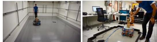
Figure 6: The ORBIT facility and the ROOTLESS platform, two means to recreate low-gravity
