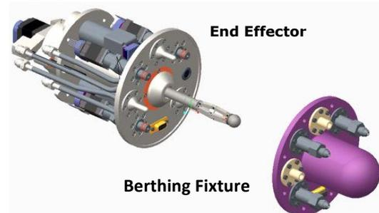
Figure 4: The ASSIST system, with its end-effector (to be mounted to a tanker satellite) and the berthing fixture (to be part of a serviceable satellite)
