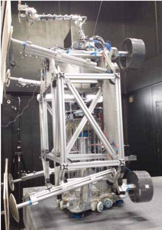
Figure 3: Testing landing and sampling on simulated Phobos gravity (courtesy of CBK-PAN)
