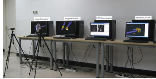
Figure 3: The hardware of semi-physical vision simulation system
