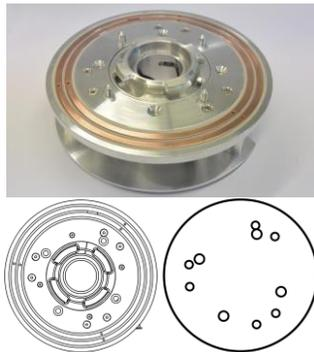
Fig. 8: Top: Multifunctional interface for coupling of individual satellite cubes. Taken from [7]. Bottom left: 2D model with view from the top. Bottom right: Final 2D edge representation for shape-based matching.
