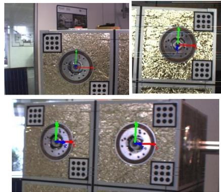
Fig. 7: Satellite modules with localized interfaces.
