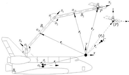
Figure 1: Free-floating flexible space-based robot
