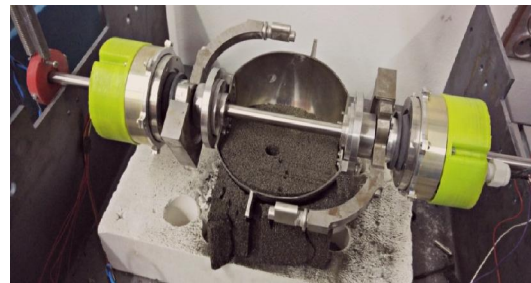
Figure 8: Breadboard with active BLDC drive
