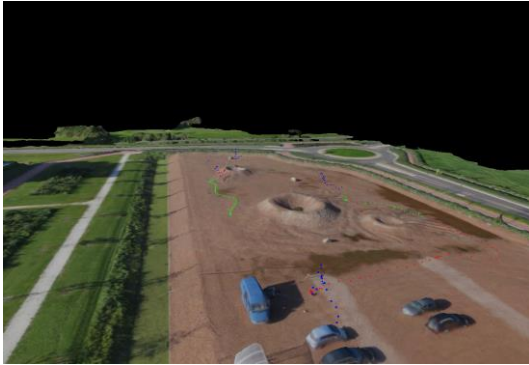
Figure 8 3D reconstruction of the DECOS test area. The trajectory of the rover –as measured by the RTK GNSS– is annotated.
