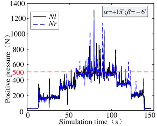
Figure 12: positive pressure of the track
