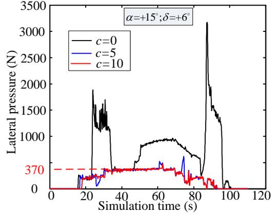
Figure 13: Lateral pressure of the left guiderail change with  $c$
