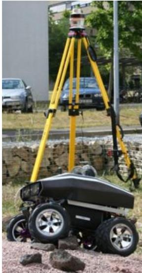
Figure 5: The MERLIN test vehicle with sensor suit for obstacle detection and avoidance in front of a precision tracking system component.
