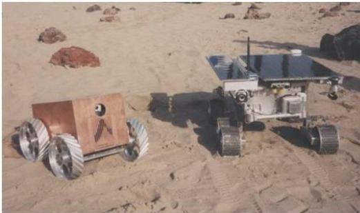
Figure 2: The small planetary rovers MIDD (developed for ESA) and Rocky VII (from JPL/NASA) during training for Mars environment.
