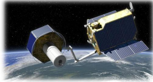
Figure 3: The DEOS scenario, where the servicer satellite with robot arm approaches the in-operational satellite at the left (image courtesy of DLR).
