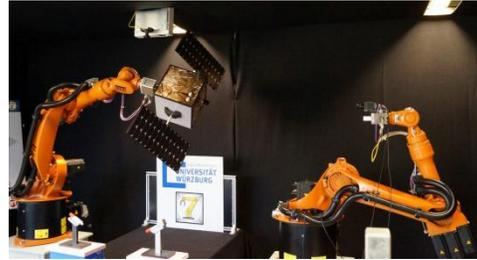
Figure 6: Robots simulating the relative dynamics in rendezvous & docking of the servicer's 3D-camera (right) to a defect spacecraft (left).
