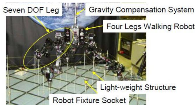
Figure 9 The JAXA four-legged robot
