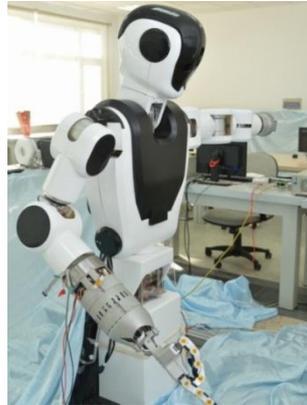
Figure 14 The prototype of space humanoid robot
