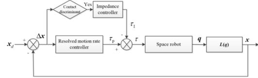
Figure 1: Block diagram of the combined control strategy.
