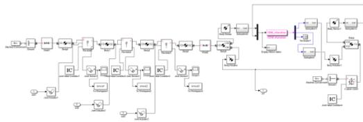
Figure 3: Block diagram of the simulation system for the robot to perform capturing task.
