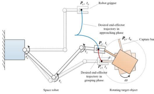
Figure 2: A 3-joint planar manipulator capturing a rotating target object.
