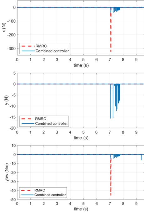
Figure 6: Contact forces and torques between the end-effector and the target object.
