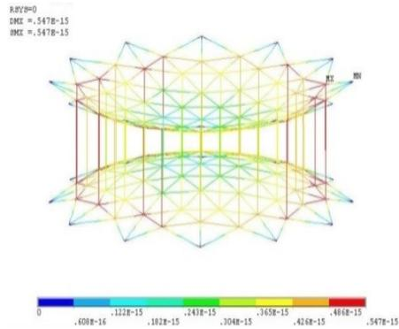
Figure 7 Deformed cloud of cable net system under pre-stressed
