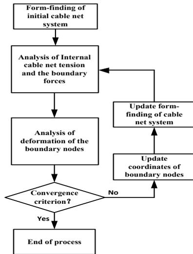
Figure 8 Iterative process of form-finding with boundary deformation
