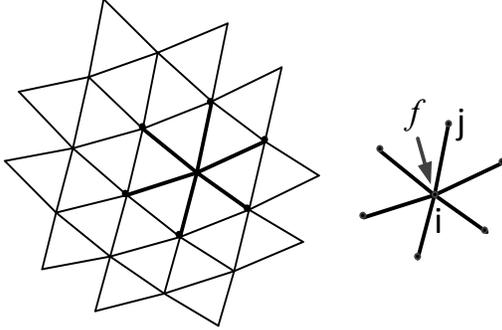
Figure 2 Part of a cable net
