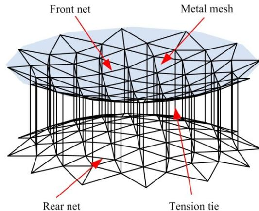
Figure 1 Composition of the cable net reflector
