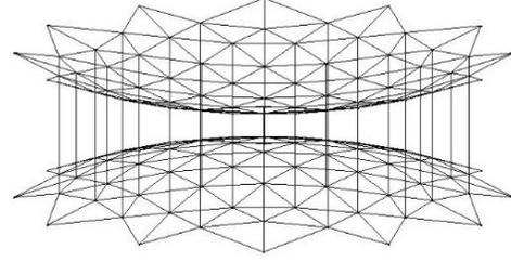
Figure 3 Multi-pivot six ring cable net
