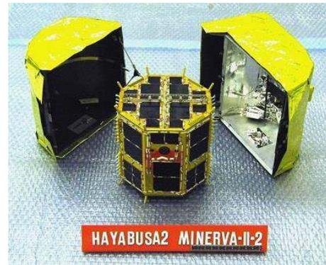
Figure 1: Flight model of the MINERVA-II2 system
