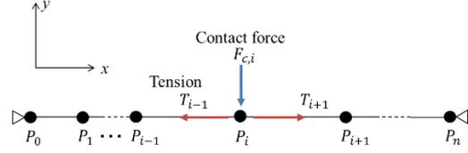
Figure 5: 2D model of the snare wire
