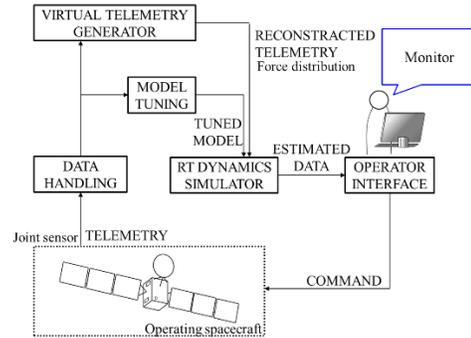
Figure 3: Framework for real-time dynamics estimation
