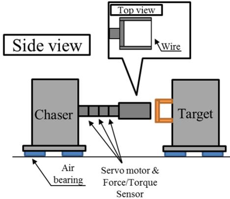
Figure 9: Ground experiment facility
