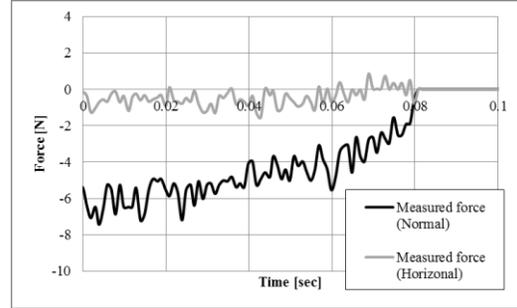
Figure 11: Obtained telemetry data about tip force
