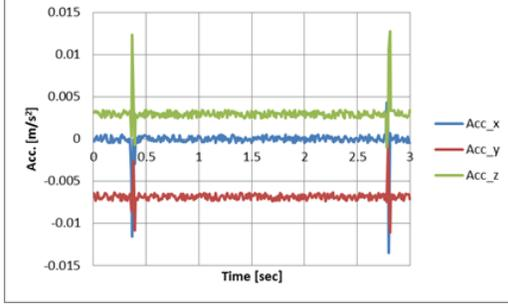
Figure 4: Simulated reaction acceleration happed by HTV's contact
