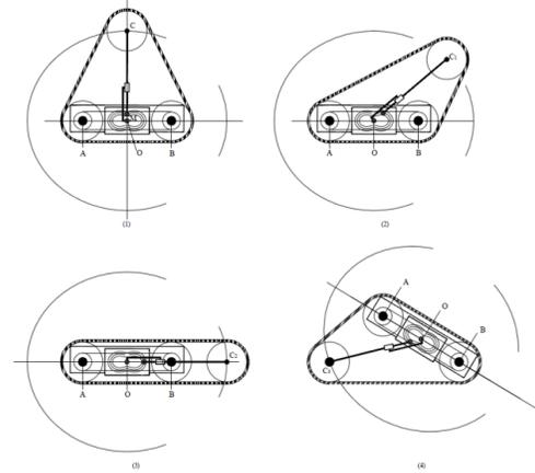
Figure 5: Variable configurations of the robot
