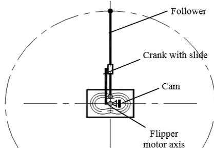
Figure 1: Schematic diagram of the track configuration-controlling mechanism, i.e. the flipper
