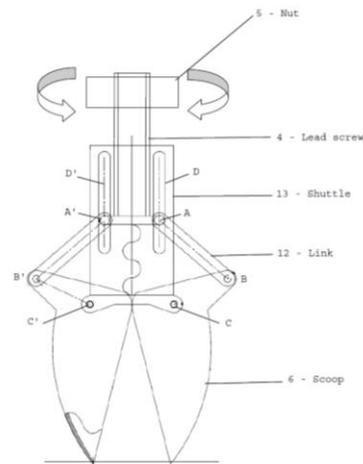
Figure 8: Scooping mechanism schematic
