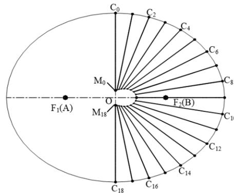
Figure 3: Motion trajectory of the planetary wheel center  $C$
