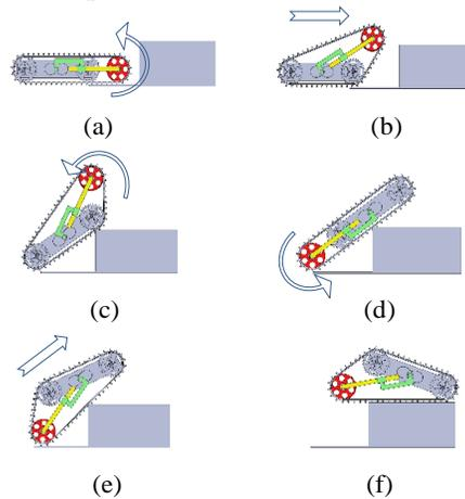
Figure 6: Rover surmounting an obstacle
