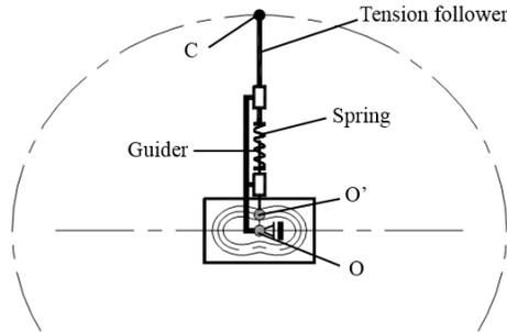
Figure 4: Schematic diagram of the track configuration-controlling mechanism with tension springs
